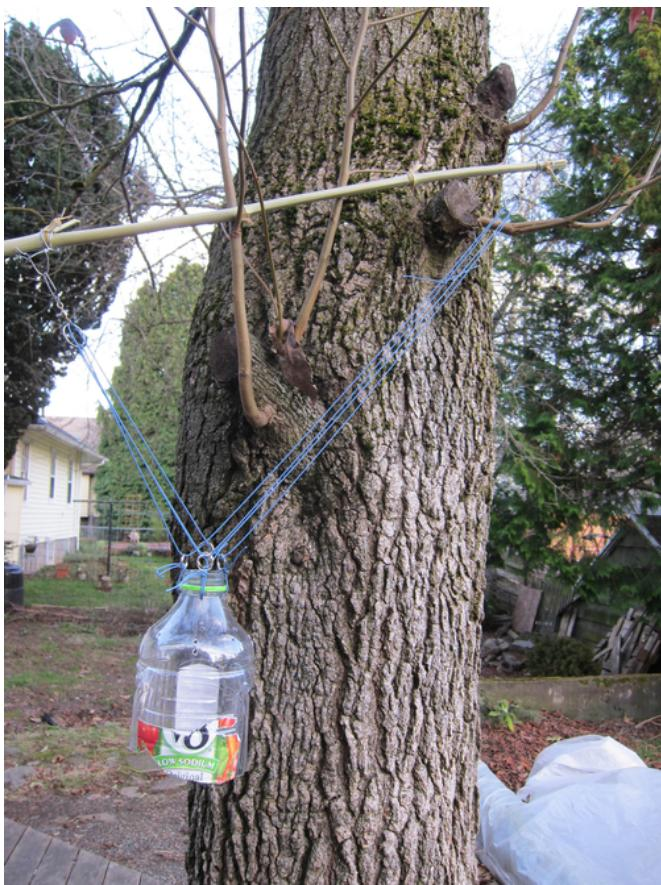
A Picavet rig is a very common type of KAP/BAP rig, I've added it to the juice bottle in a fairly simple way, using 1/2" key rings.
