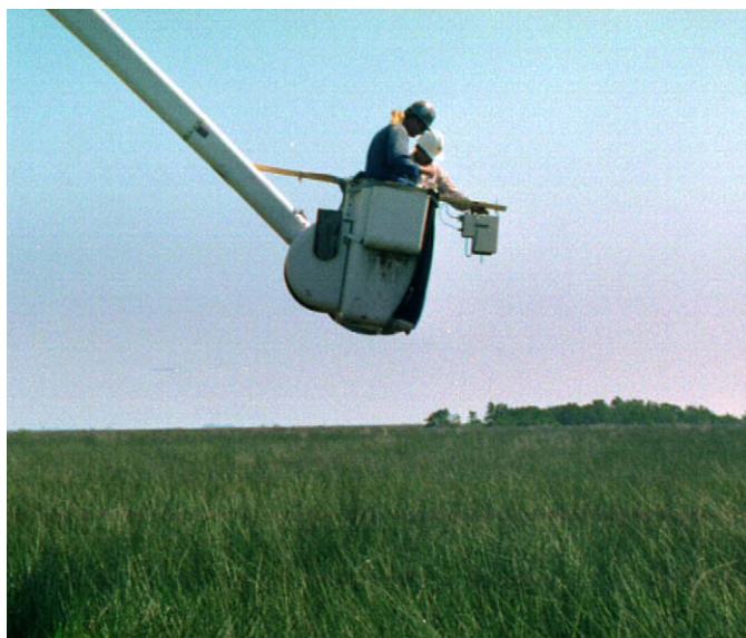
Fig. 3. Collection of spectra above the canopy of salt marsh in Pascagoula, Miss., with the GER 2600.
