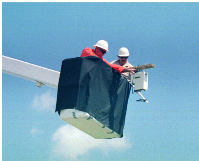
Fig. 4. Calibrating the GER 2600 Spectrometer using a Spectralon (Labsphere, Inc.) reflectance panel, an NBS standard for reference. A dark cloth is used on the bucket to suppress scattered light.
