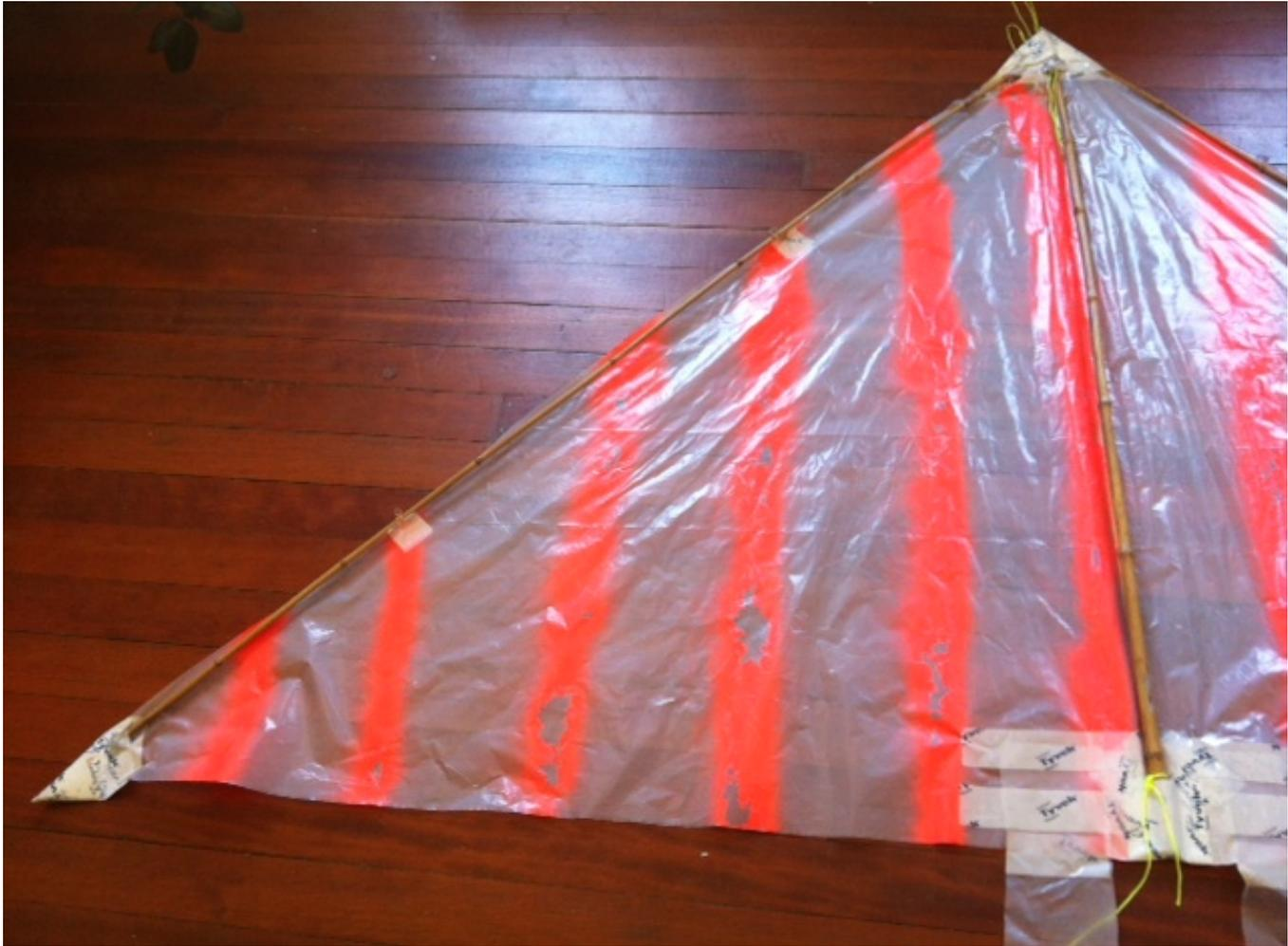
Insert the bamboo culms into the pockets, the thicker 3/4" culm for the vertical spar and the thinner 1/4" culms for the leading edge spars. I had to bend the bamboo slightly to get them into the pockets, which is helpful for keeping the kite taut in the end. Thicker ends of the culms should be in the trailing edge pockets.
