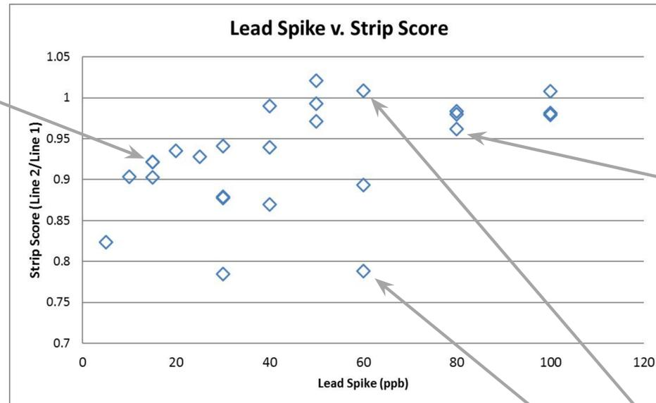
Figure 6: Computer Vision Strip Score Compared to Spiked Concentration
