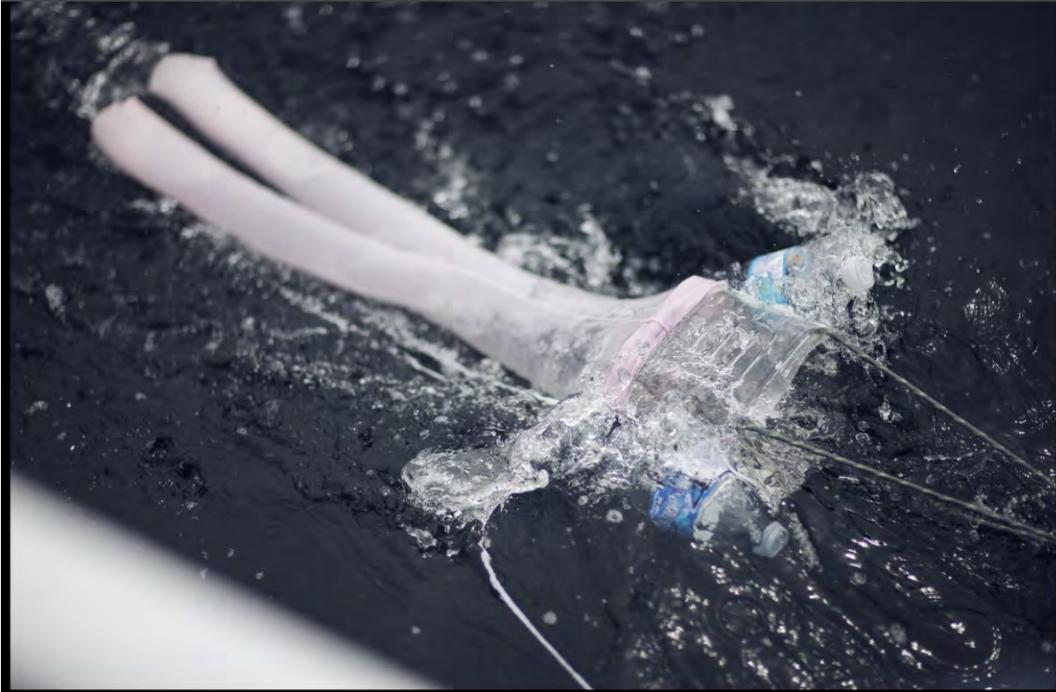
Created with baby's tights, soda pop bottles, and other inexpensive and easy to find materials, BabyLegs can be used to skim the surface of water in rivers, streams, and oceans for floating marine microplastics by hand or from a boat. This instrument is called a **surface trawl**.
