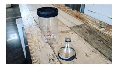
5) Place the top of the bottle inverted in the bottom of the bottle and secure it either with the binder clips or the paper clips.
